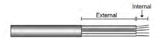
Figure 21: Insulation stripping – AC
